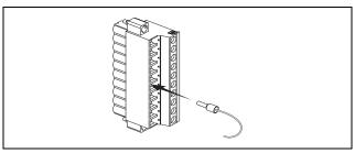
Figure 7. 10-Terminal Detachable Screw-Terminal Connector with a Ferrule
